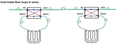
The variable time delay module selectively routes optical signals through N fiber segments having different lengths. Each fiber segment is defined to have the delay as
